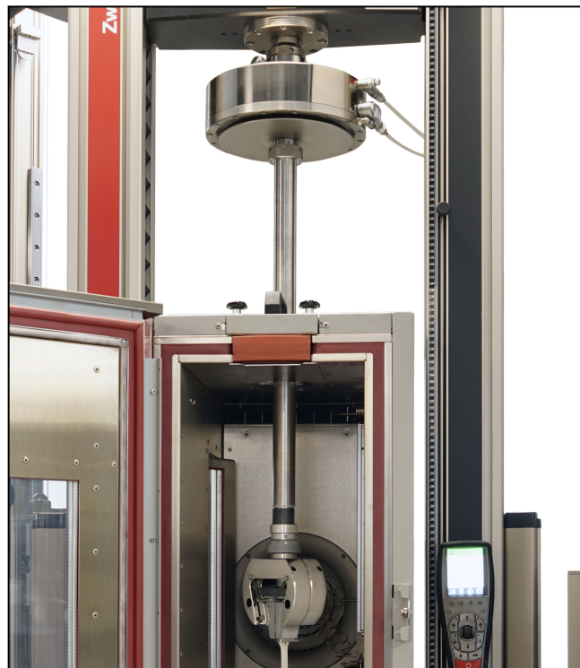
Pneumatic grips type 8304, Fmax 20 kN with pneumatic operation, temperature chamber
