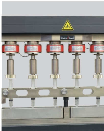
Fig. 2. Parallel testing of syringes
