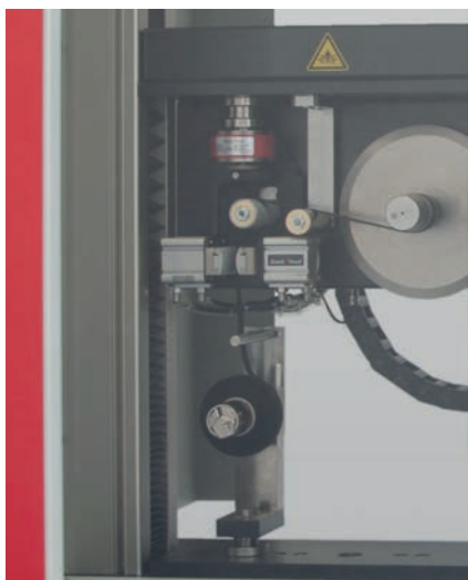
Fig. 1. Unrolling test on gauze bandages
