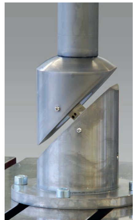
Fig. 2. Torsion test on vertebral body implant
