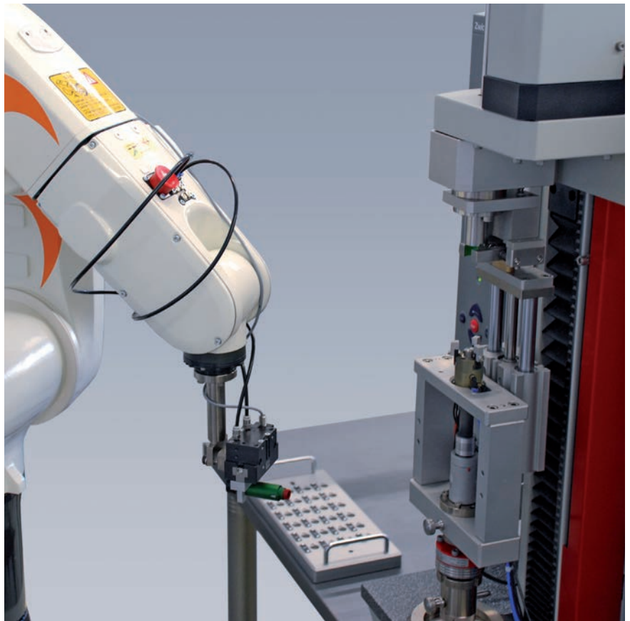
Fig. 2. Fully automatic testing system for insulin pens
