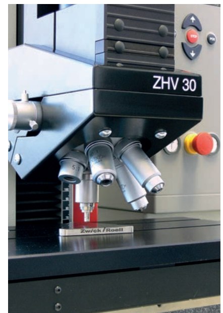
Fig. 3. Hardness test on dental ceramics
