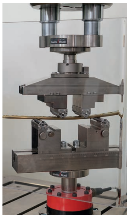
Fig. 2. Flexure test on bone plates
