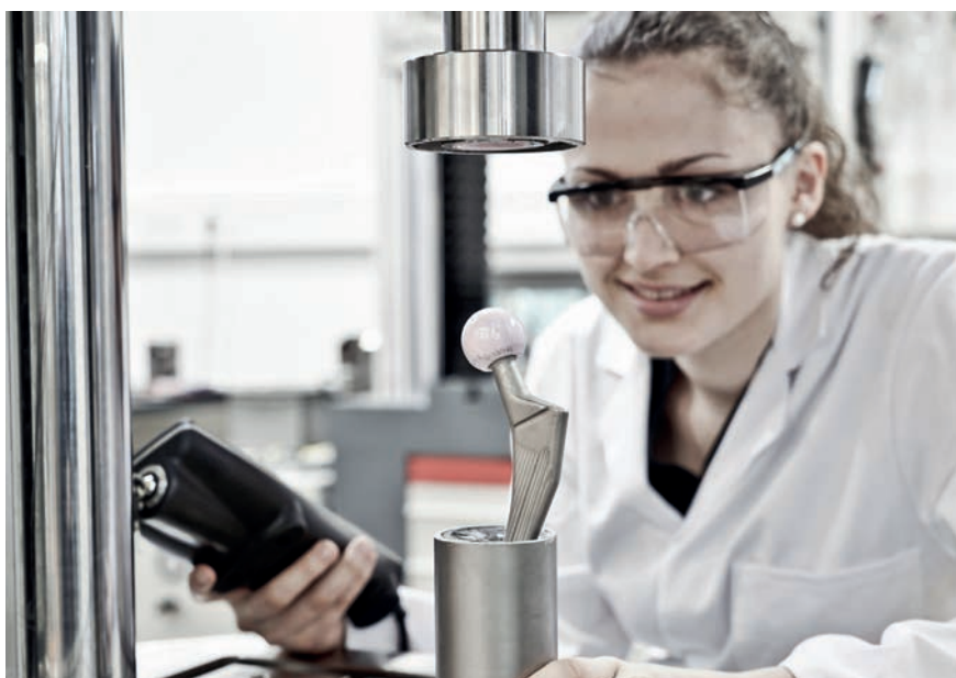
Fig. 1. Fatigue test on hip prosthesis
