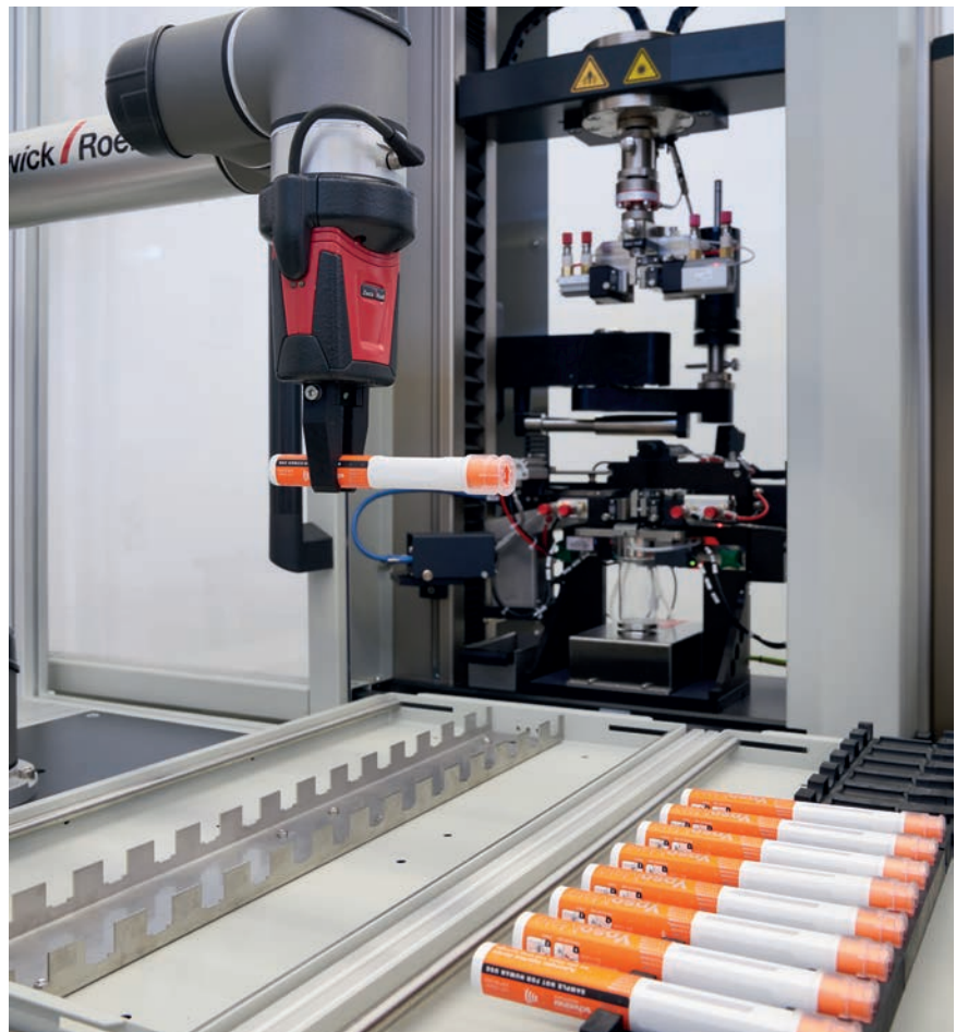
Fig. 2. Testing system with fully automated specimen feed
