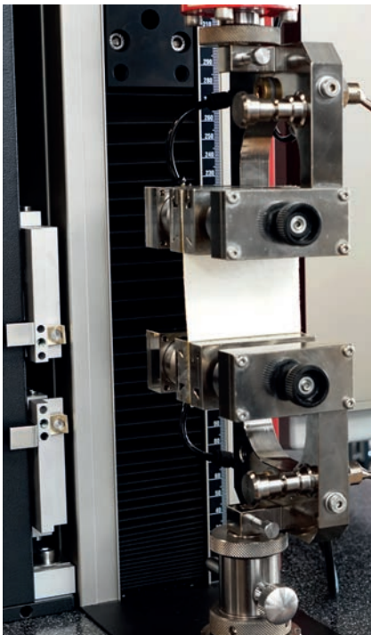
Fig. 1. Tensile test on medical textiles
