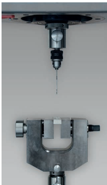
Fig. 2. Penetration test for a bone drill
