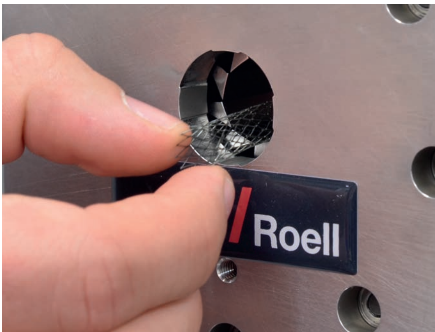
Fig. 1. Radial compression tests on stents
