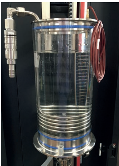
Fig. 1. Fluid bath with temperature control unit
