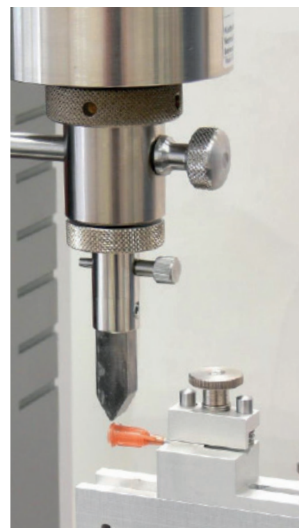
Fig. 4. Flexure test on needles
