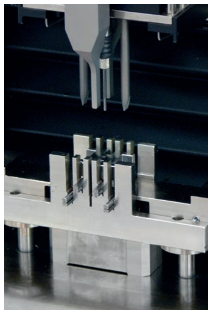
Fig. 2. 4-point flexure test on dental ceramics
