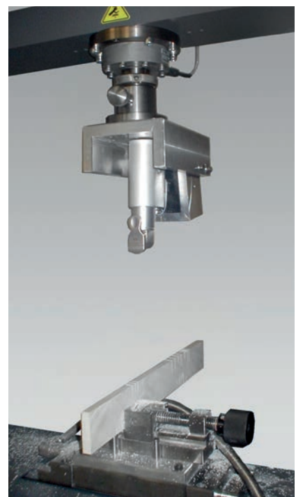
Fig. 3. Compression test on sagittal saw blade
