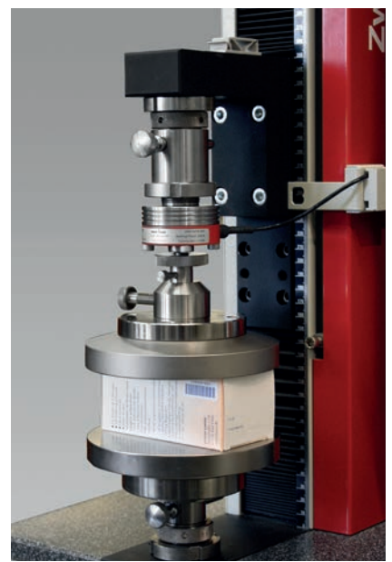
Fig. 3. Box crush test on medication packaging
