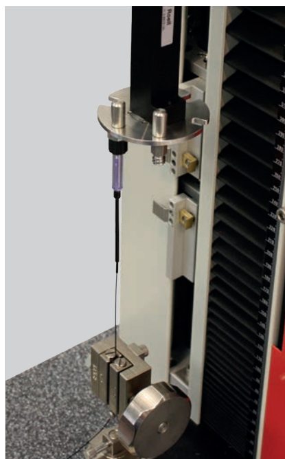
Fig. 2. Tensile test on catheter systems
