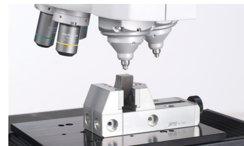
Vickers hardness tester: the turret adapts to different test methods
