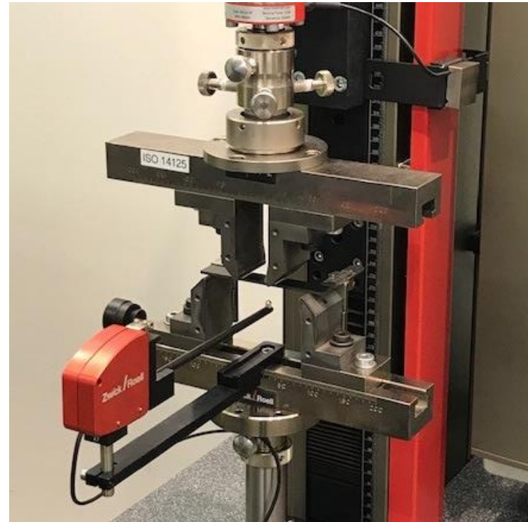
4-point flexure test middle: deflection measurement with displacement transducer T25 right: deflection measurement with videoXtens and plunger
